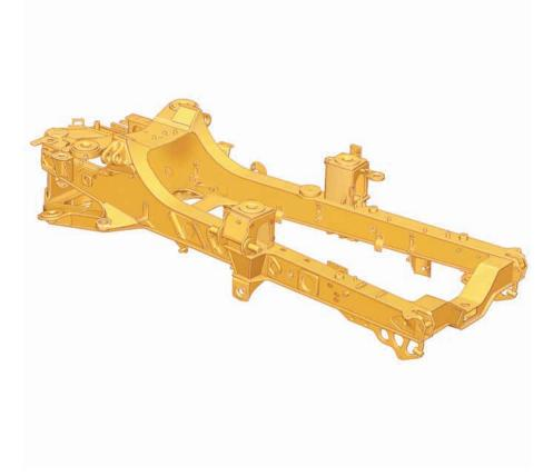
**Hitch Construction.** Two-piece hitch construction features a strong, durable cast steel head bolted to a hard wearing forged steel tube. The hitch tube has large, hardened bearing areas and a hardened thrust face for reduced maintenance and longer life.
